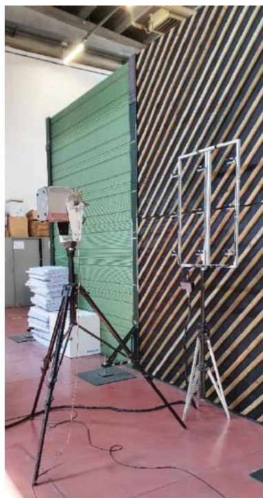
Figure 27. Laboratory reflection index measurement test on a timber noise barrier with the standard equipment for EN 1793-5. Sound source height: 2,00 m above ground.
