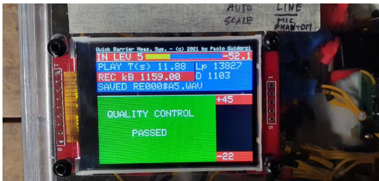
Figure 21. The control and processing unit confirming that the quality control of a measured impulse response has been passed.
