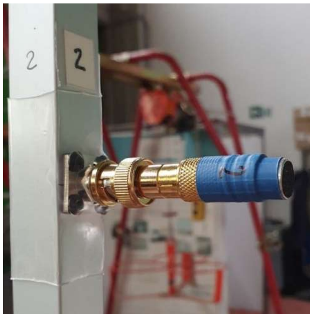
Figure 9. One out of six electret microphone mounted on a vertical aluminium stick.
