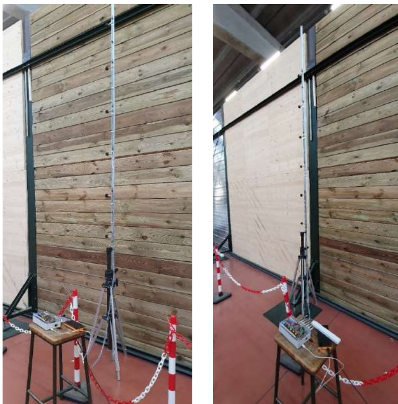
Figure 29. Laboratory sound insulation index measurement test on a timber noise barrier with the new equipment. Left: across the acoustic elements. Right: across a post. Sound source height: 2,00 m above ground.
