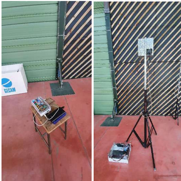
Figure 17. Wireless transmitter/receiver system connected to the control and processing system (left) and to the UNIBO lab-made lightweight loudspeaker (right).
