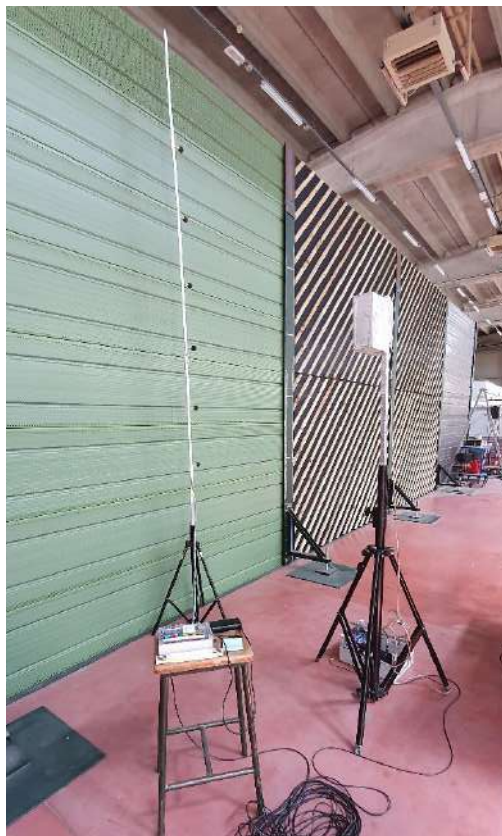
Figure 40. Laboratory reflection index measurement test on a metal noise barrier with the equipment for the new quick method. Sound source height: 2,00 m above ground.
